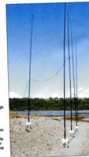
Figure 5 — The cat was kind enough to empty several more buckets of litter so more elements can be added. Using 20 meter data from Table 1, I measured and cut the wires needed for a reflector and two directors. I've included additional data for other bands these verticals could support. Part of the 20 meter reflector wire is extended above the pole and the other couple inches hangs down toward the ground.
