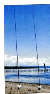
Figure 3 — The coax support vertical is built next. It gets the coax away from the driven element's bottom section. The coax support vertical is built just like the driven element. Each section is raised in section as they are extended, until both are at full height. At this point you have an omnidirectional half wave vertical dipole. This is a good time to hook up the radio and check the band to see where you want to aim the antenna.
