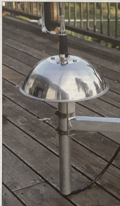
The Mixing Bowl Special with its gleaming steel ground plane.
