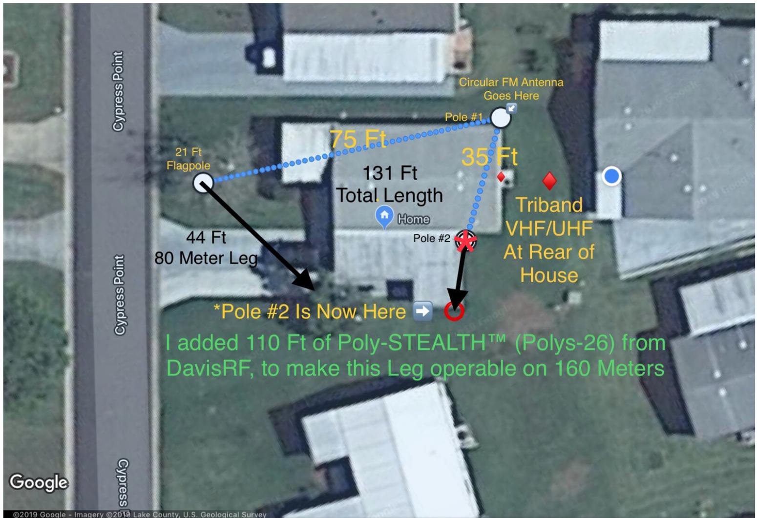
I added 110 Ft of Poly-STEALTH™ (Polys-26) from DavisRF, to make this Leg operable on 160 Meters
