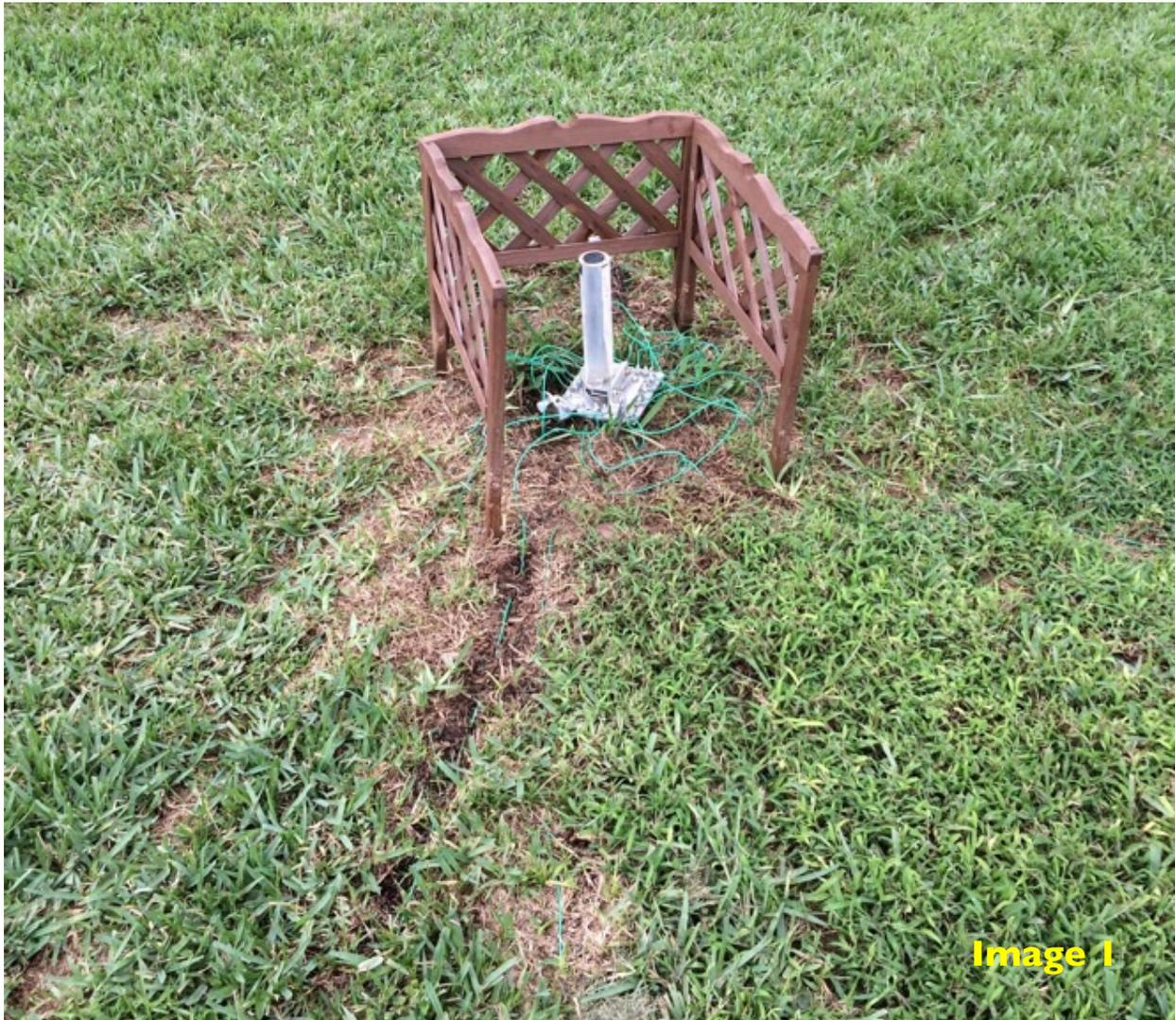
This is my “Refurbished and Reconfigured Force I2 Flagpole Vertical.” I replaced the OCF section and a damaged section at the top. This “21” configuration is designed to be bottom fed. I removed the paint on the bottom to accommodate the tilt over bracket that also doubles as the feed point. The bracket then mounts to the PVC insulated mounting pipe. (Img. 1)
