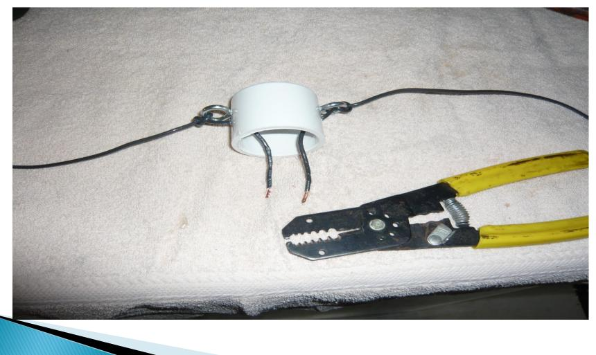
Crimp a eye lug on the wire closest to the screw with 2 nuts. Make sure that this is a solid connection. Put the ring on the screw and tighten the nut.
