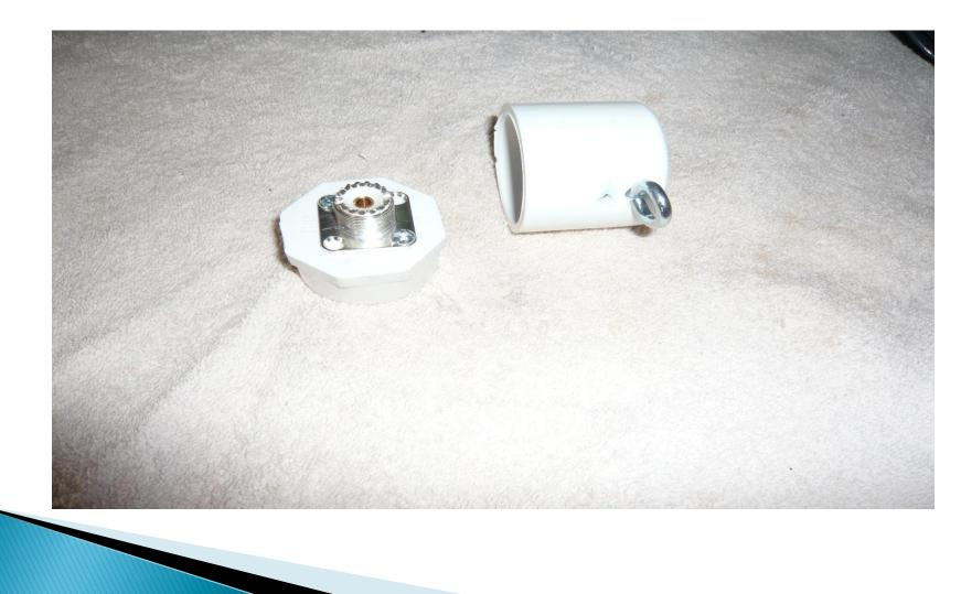
Take the precut wires and run them through the eyebolts and tie a knot. Leave just enough to feed through the hole and extend the bottom of the cap by an inch. Strip each wire <sup>1</sup>/<sub>4</sub>"
