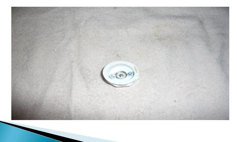
Get the eyebolts and nuts. Drill 2 holes opposite each other in the rounded cap. Drill another hole just below the eyebolt for the antenna wires to enter.
