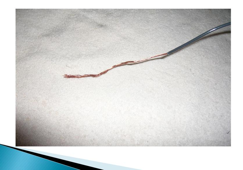
Insert the stripped end into the insulator about  $\frac{1}{2}$  way. Make a wireman's twist on the wire to form a tight connection. Solder these connections for strength and conductivity.
