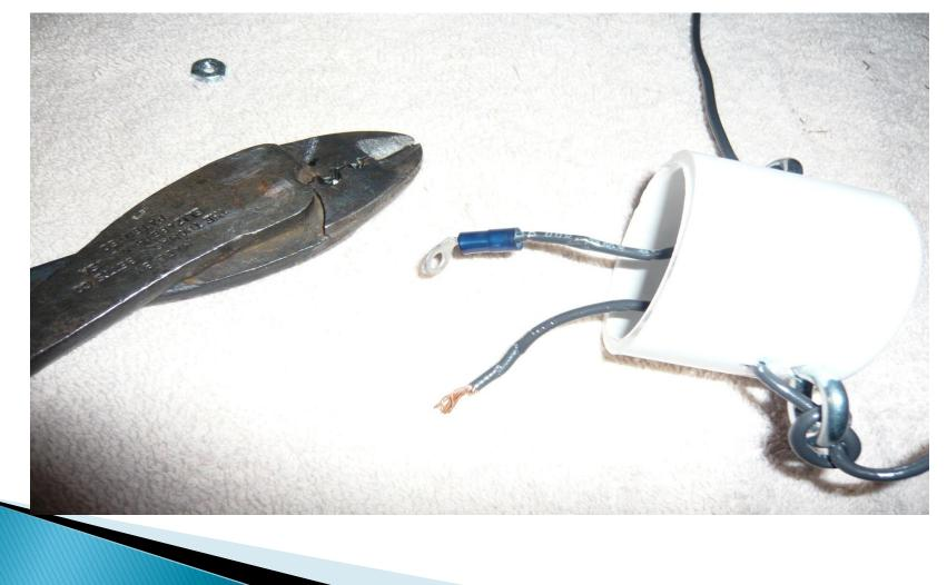
Insert the other antenna lead into the center post of the connector. You may have to trim the wire to fit. Solder this connection. Be careful not to use to much heat.
