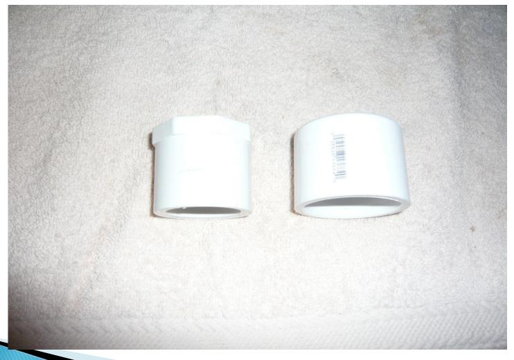
Note that the plug and cap are about the same length, not good. Cut about <sup>3</sup>/<sub>4</sub>"" off of the flat plug. This will give more working room.
