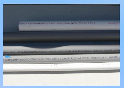
A piece of scrape 1-1/2" plumbing PVC pipe A piece of scrap 3" plumbing PVC pipe The schedule 80 2" pipe was \$6.47 per 10' The 2-1/2 schedule 40 was \$7.04 per 10'
