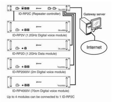
box plugged into the controller is referred to as a 'Module' or 'Node', and then you have the Controller which controls the whole stack and that reports to the Gateway for orders. (Hence you see why the term 'Stack' is used)
