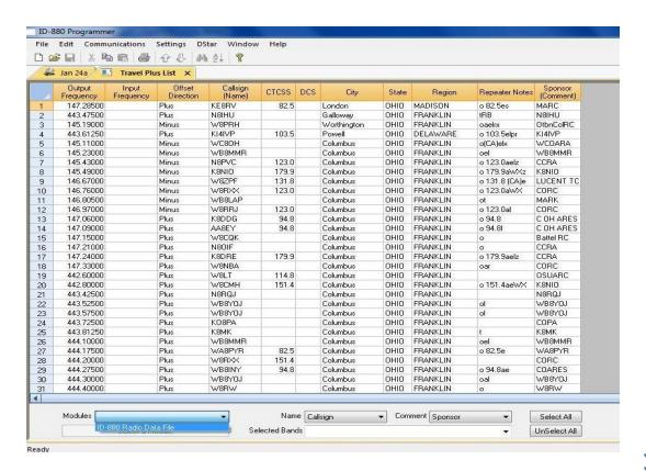
At the lower left of this tab is "Modules". Click the drop down and 'ID 880 Radio Data File' will appear. Next the tab below will have Create Files for ID800. Select this entry.
