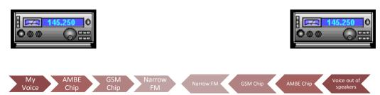
In DV (Digital Voice mode) your voice goes through the Advanced Multi-Band Excitation (AMBE) chip where it is encoded digitally plus text, and any other data, into GSM (the same process happens in cell phones) then stuffs it out the Antenna as Narrow FM.
