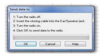
Connect the cloning cable to the USB port on you computer. Then follow the above directions.
