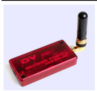
This is pretty new to the market. It works as a hotspot. Basically it works similar to a DV-Dongle except you don't use a head set and mic, you use a D-Star radio. It has a 10mW (that's milli watt) radio inside that works on a simplex frequency. So if you want to use your D-Star radio, but no repeaters around you can use this to get you out similar to a DV Dongle. So all of the limitations with DV-Dongle, just you can use a D-Star radio to go in and out.
