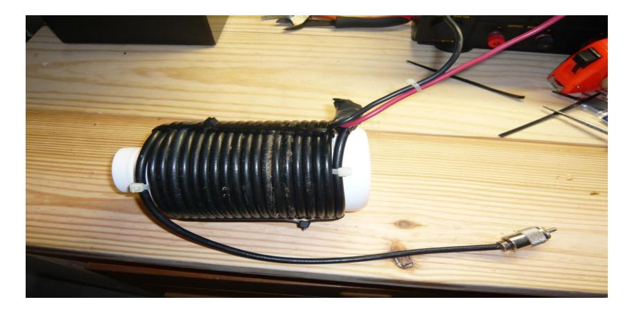
Now wrap the cylinder with the coax evenly. Do not leave any gaps and do not cross **OVEr** the wire. Secure the coax at the end with another ty-wrap that goes through the cylinder.
