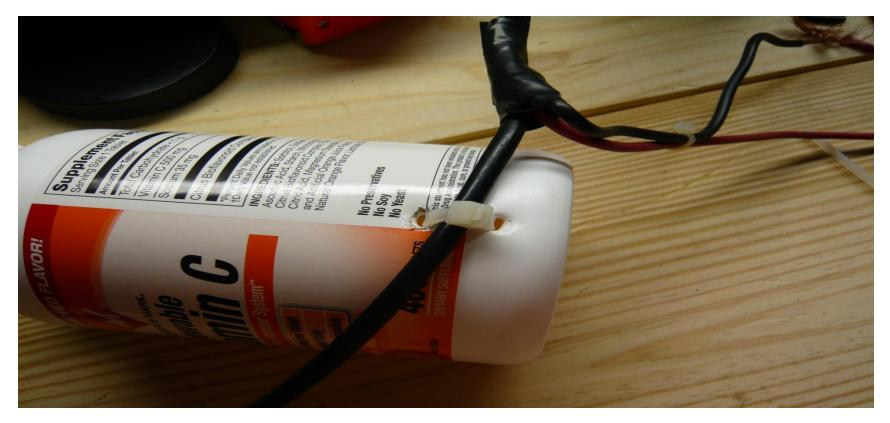
Now it is time to secure the end of the coax to the cylinder. Leave approximately 1" of coax past the ty-wrap and tighten securely.
