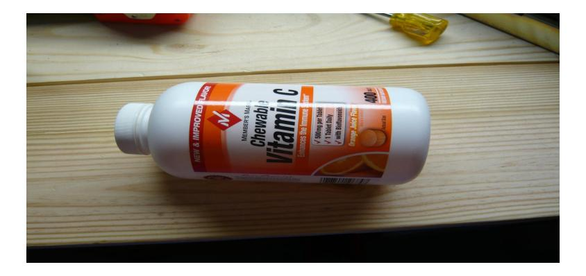
Locate a pill bottle or other non-conductive cylinder or piece of PVC pipe at least 3" in diameter. I used my XYL's vitamin bottle . I put the pills in a sandwich bag.
