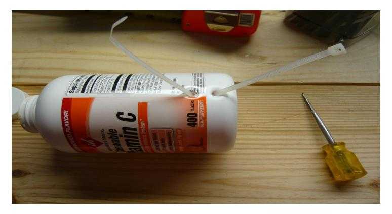
Punch or drill 2 holes near one end about an inch apart from each other. Insert a tie wrap or string thru one hole and out of the other hole. This will secure the coax.
