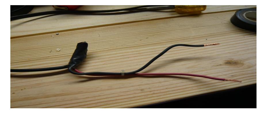
Solder and tape the connections. Remember which is the center conductor and which is the ground. That is why I like black and red. This is the Villages after all.
