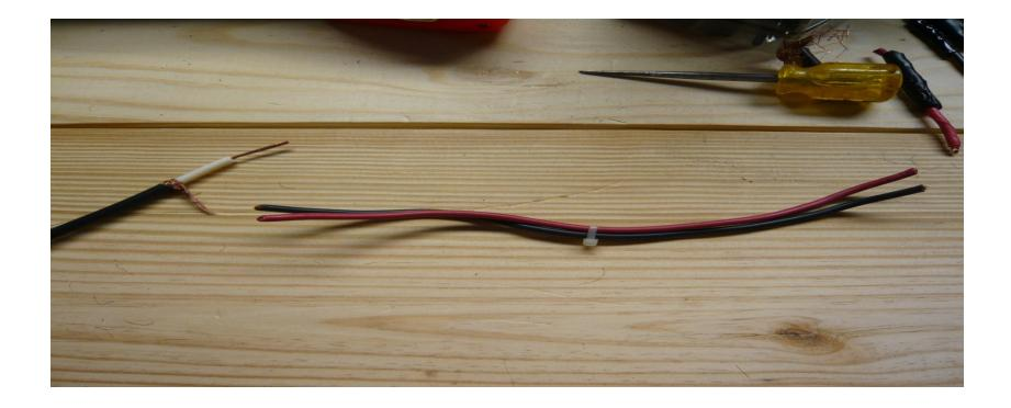
Prepare the end of the coax as shown., to be soldered. Locate 2 pieces of wire 16 to 14 AWG, about 8" long.
