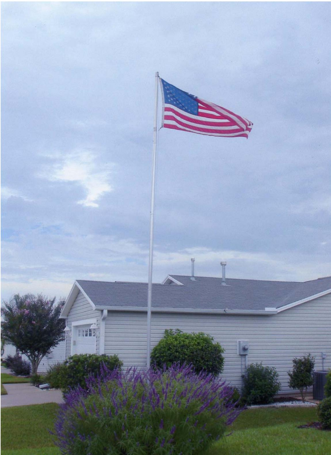
**This installation has a flagpole antenna set in a “well” surrounded with flowers. The “well” is lined with brick and has the mounting for the pole and an auto tuner wrapped in a trash bag (tuner is waterproof). The “well” is filled with pea gravel for drainage, covered with lava rock and surrounded with flowers. This is what it looks like—look hard through the flowers and see if you can make it out?**
