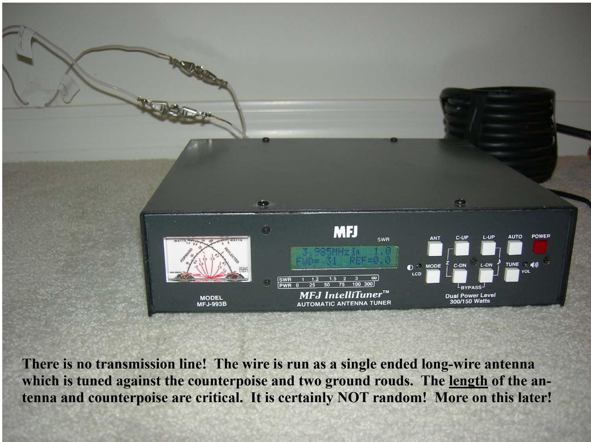
**There is no transmission line! The wire is run as a single ended long-wire antenna which is tuned against the counterpoise and two ground rouds. The length of the antenna and counterpoise are critical. It is certainly NOT random! More on this later!**
