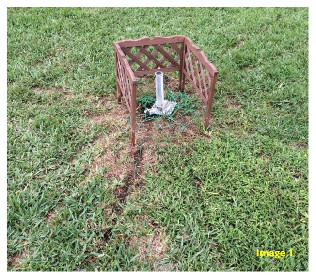
This is my "Refurbished and Reconfigured Force12 Flagpole Vertical." I <u>replaced</u> the OCF section and a damaged section at the top. This "21" configuration is designed to be bottom fed. I removed the paint on the bottom to accommodate the tilt over bracket that also doubles as the feed point. The bracket then mounts to the PVC insulated mounting pipe. (Img. 1)
