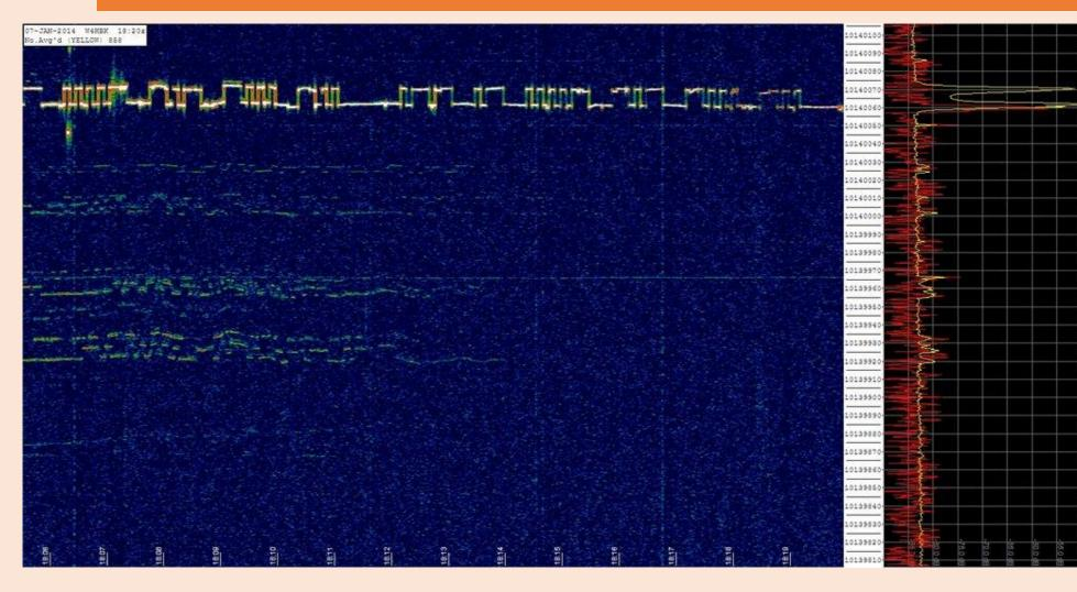
This a picture of the arrival of the XRAY emission of a Solar flare. When this happens, the D layer of the ionosphere ionizes and skywave signals are totally attenuated. This is a 10 minute view showing the period of this effect and you can see the distortion of the E and F ionospheric layers as the earth is hit by the XRAY emission from the solar flare.
