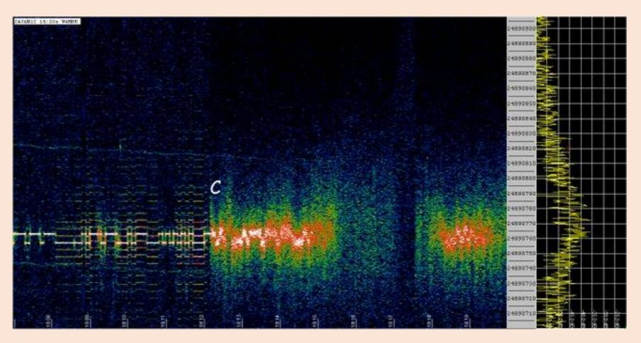
This is a 10 minute display of my signal on W4HBK's grabber. The multiple signals appears in the first 4 minutes of the picture. There is not a known explanation of how this happens. Then my signal is greatly amplified and distorted by the ionosphere for the rest of the screenshot. I can't explain what is going on to cause this screenshot other than the only times these effects have been seen are during a Coronal Mass Ejections from the Sun.
