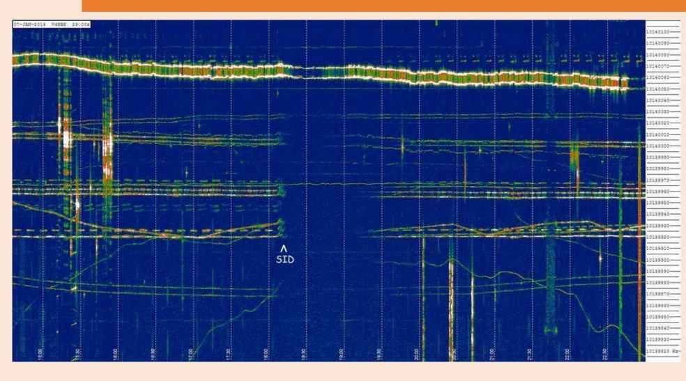
This is the 8 hour picture of the same solar flare. It shows the length of the D layer ionization and attenuation of the skywave signals arriving at W4HBK's grabber. As you can see the period was from about 18:10Z to 19:20Z. You can also see more clearly some attenuation of WA4KBD's signal but that it was still visible through the total blackout period but all the New Mexico signals were totally gone.
