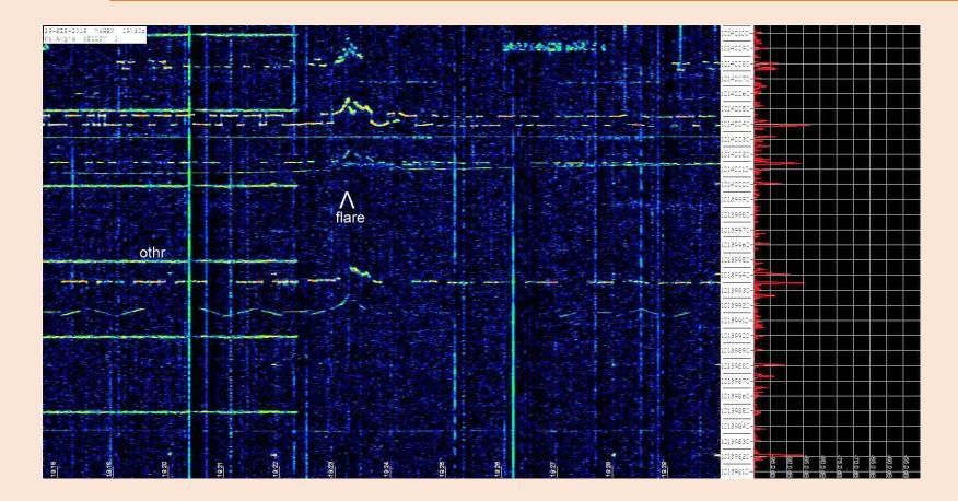
This is a screenshot of the arrival of a Coronal Mass Ejection of particles from the Sun. When it comes in contact with the ionosphere it causes it to distort. Radios signals that arrive the ionospheric layers are distorted. This picture shows some of these distortions. (this is my favorite and most interesting part of QRSS. Most signals are from New Mexico as copied in Florida.
