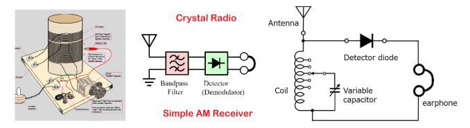
The CRYSTAL receiver uses an LC "tank" to selected frequency and a diode to demodulate the signal.
