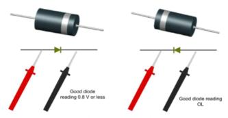
Figure 6: Reversing the red and black probes allows you to check the forward and reverse bias conditions of the diode. [QS1710-Danzer07]
