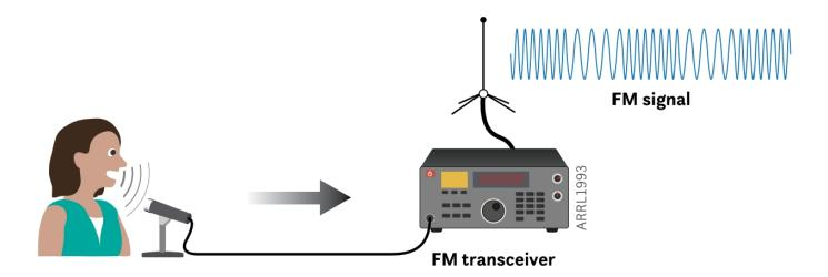
Figure 2: In this example the operator is speaking into the microphone of an FM transceiver. Look at what happens to the output signal's frequency as she speaks. Notice that the horizontal distances between the waves keep changing. This means the frequency of the signal is changing while the power remains constant.
