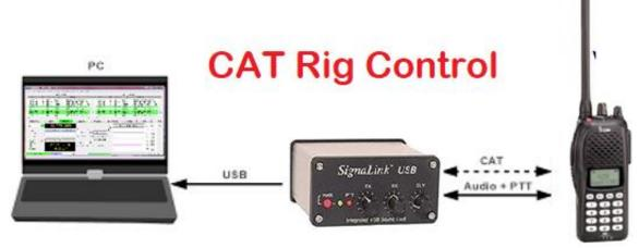
Rig control via CAT (Computer Aided Tuning) allows a computer to control functions of a transceiver just you would operate and read the displayed information. The audio input and output of your transceiver are connected to a computer sound card to produce the digital modulations such as APRS, Packet or FT8.
