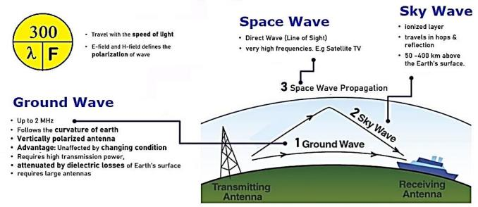
**The ionosphere** is the part of the atmosphere that enables the propagation of radio signals around the world.
