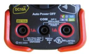
Figure 2: The center black jack is used as the return for measuring the items listed above the right-hand red jack, plus low-current dc. The left-hand red jack is used only for high-current dc.
