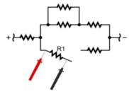
Figure 5: Resistance is measured with one end of the resistor disconnected from the circuit. [QS1710-Danzer06]
