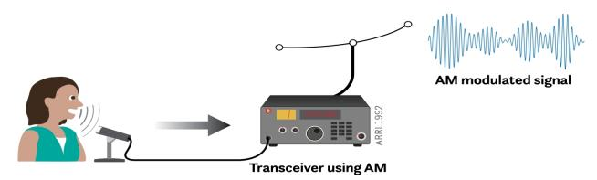
Figure 1: AM signals are amplitude modulated, which means that the signal amplitude, or strength, changes rapidly along with your voice. Notice how the heights and shapes of the waves in the output signal are changing. Look closely, however, and you'll see that the horizontal distances between one wave and another never change. This means that while the amount of power in the signal is changing, its frequency remains the same.
