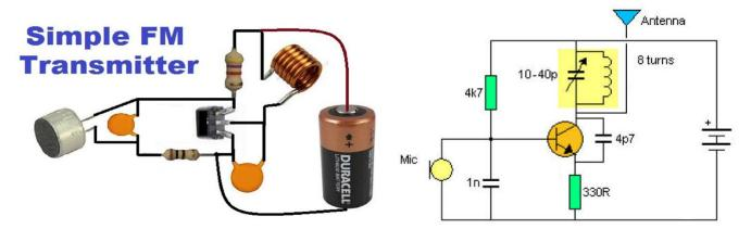
A simple FM TRANSMITTER is an LC oscillator for a specific frequency plus a condenser microphone (capacitor microphone). The sound waves change the microphone's capacitance in the LC "tank" oscillator to produce FM.
