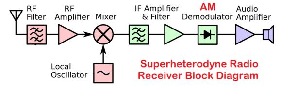
The **SUPERHETRERODYNE** receiver mixes the selected frequency with an oscillator to produce an IF (difference) and a diode to demodulate the signal. This combination provides improved SELECTIVITY and SENSITIVITY.
