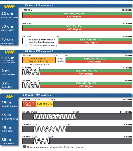
Technician Licenses may use up to 1500 Watts PEP on the VHF and higher bands, but are limited to 200 Watts on the HF bands.
